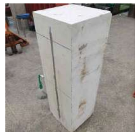
(e) After NSM strengthening
