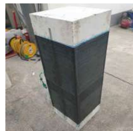
(f) After FRP-sheet reinforcing
